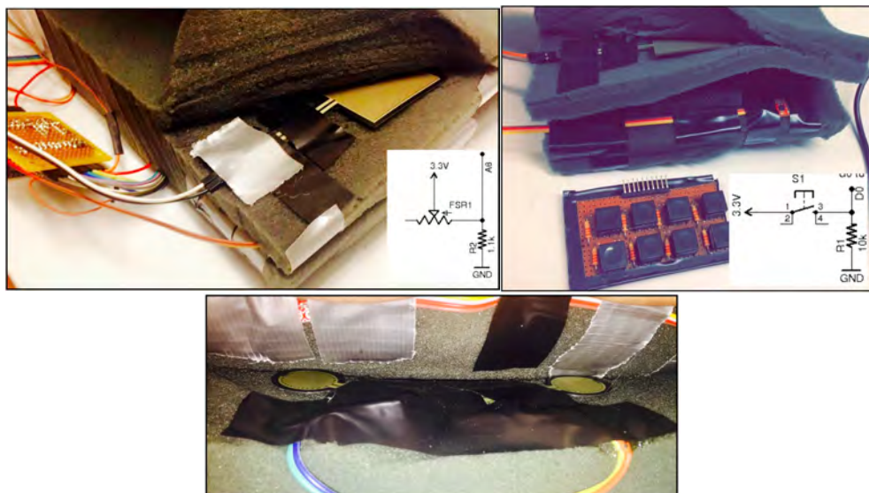
Fig. 3. FlexSynth – inside the FlexSynth Left – large FSR, Right – switch matrix and IMU, bottom – small FSRs (slide bar)
