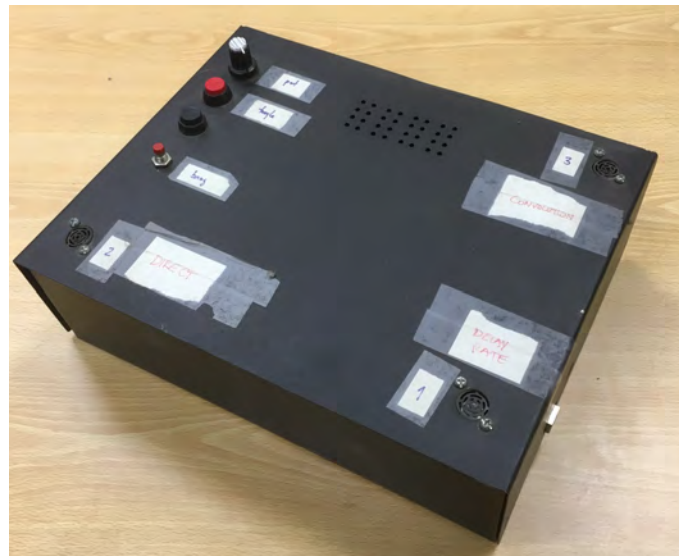
Fig. 1. The AirTouch, instrument especially developed for iCons. This instrument contains three ultrasound distance sensors (labeled 1, 2 and 3 in the picture), a knob, two toggle buttons and a trigger button. The device contains an Arduino board and connects to a computer via a USB port.
