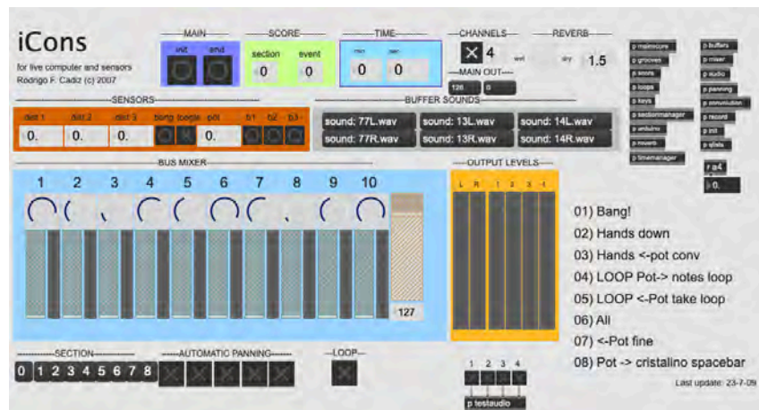
Fig. 2. MaxMSP patch. AirTouch data is displayed in the orange box. The patch also displays sounds currently being triggered, audio output levels, time, and section number. An abbreviated score is displayed in the bottom right corner.
