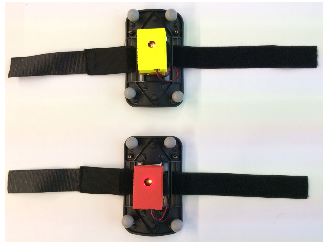
Figure 2: Rigid plates with retroreflective markers and custom boxes (coloured) containing the IMU units.
