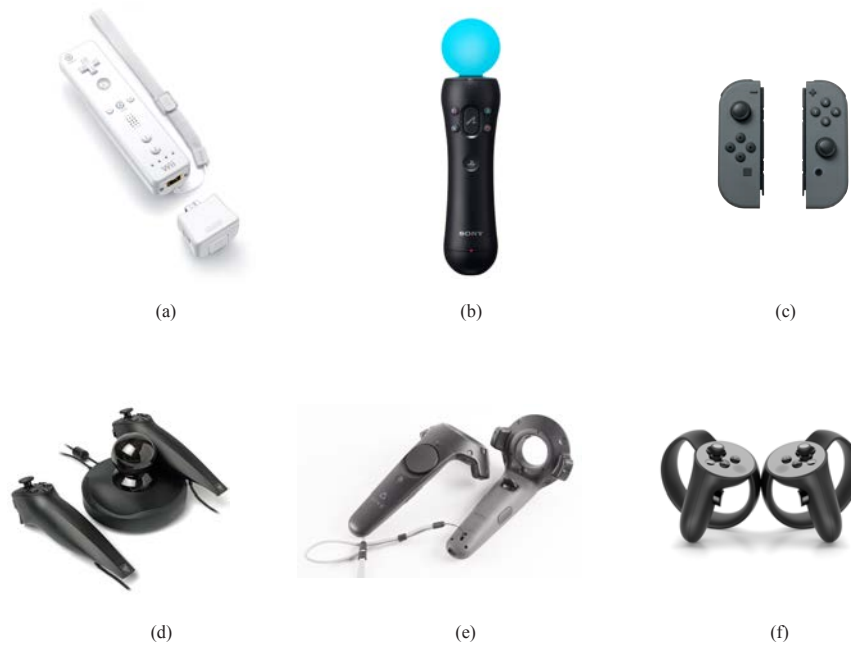
Fig. 1 Handheld motion controllers: (a) Wii Remote with Wii MotionPlus expansion; (b) PlayStation Move; (c) Joy-Con; (d) Razer Hydra; (e) Vive Controller; (f) Oculus Touch.
