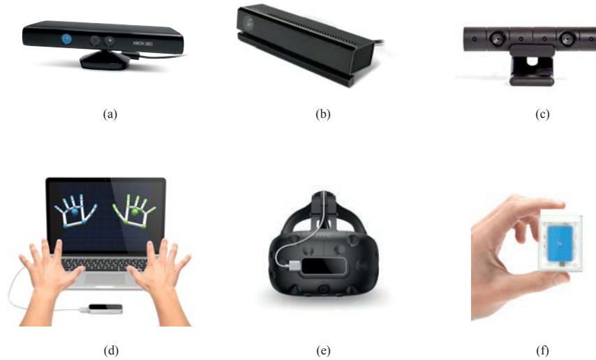
Fig. 2 External Camera-like Motion Controllers: (a) Kinect (version 1); (b) Kinect (version 2); (c) PlayStation Camera (2016 version); (d) A Leap Motion Controller used as a tabletop device with a laptop; (e) A Leap Motion Controller mounted on a head-mounted display; (f) Soli Development Kit.
