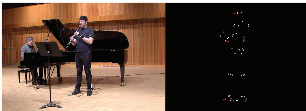
FIGURE 3 | Frame of the right-side camera video feed and corresponding motion data frame showing point locations. The markers in red were used for feature extraction.
