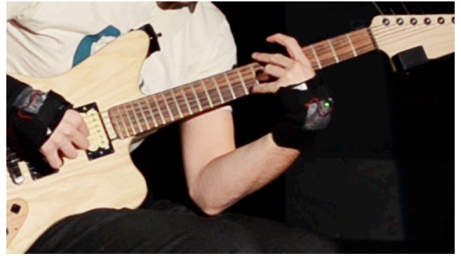
Figure 1: Use of wearable sensors: flex sensors placed on the wrist activated by a sound-facilitating support gesture.
